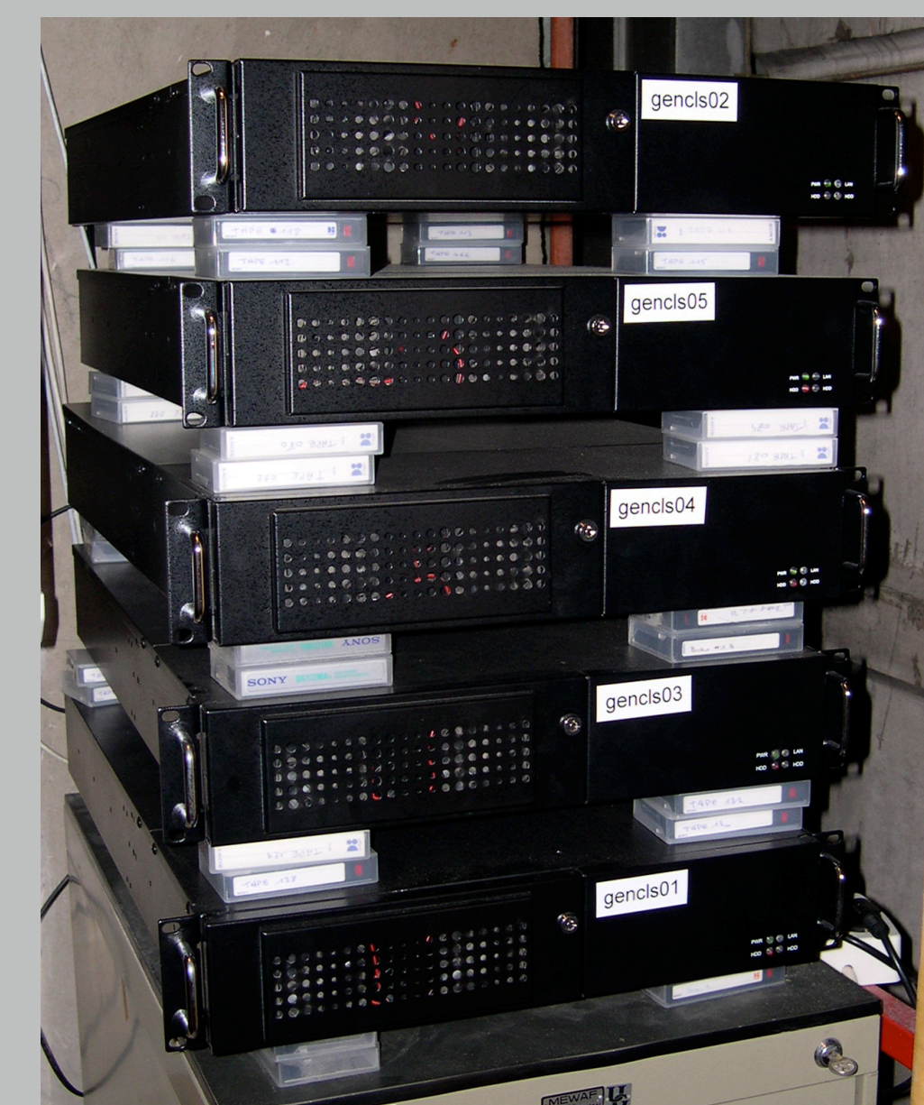
A picture of the 5 nodes of Hagrid. These are the 5 “pizza” boxes (2U). Each one has 2 AMD processors and 1 Gb of RAM.
